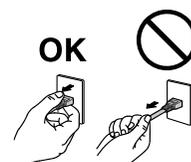
**The equipment must be connected to a grounded main outlet.**
